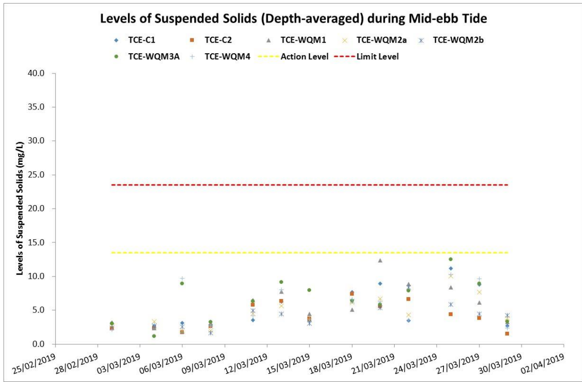
Figure 7: Levels of Suspended Solids (Depth-averaged) (mg/L) recorded at Mid-ebb Tide during the Water Quality Monitoring between 1 and 31 March 2019
